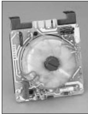
Replaceable plug-in circuit cards simplify field repair of the TF-3AC flasher/lampchanger. Left, power control circuit. Right, flash code timer.
