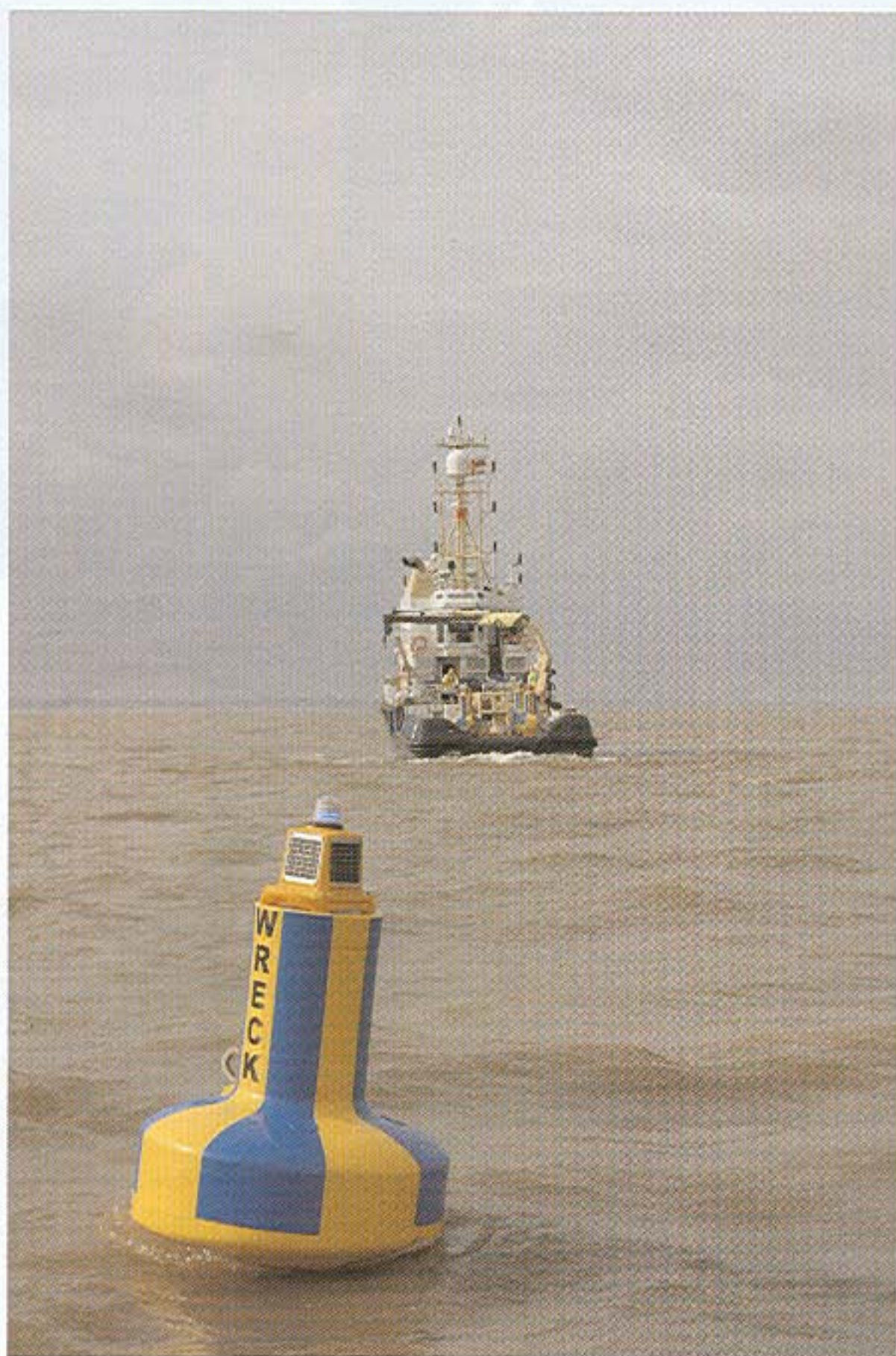
The Trinity House Rapid Intervention Vessel Alert deploying an emergency wreck marking buoy in the aids to navigation trials area off Harwich on the east coast of England. Other emergency wreck marking buoys are to be seen on the vessel's working
