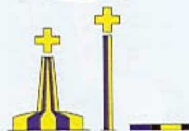
This drawing from IALA Recommendation O-133 illustrates the colours of the buoy body, superstructure and topmark.
