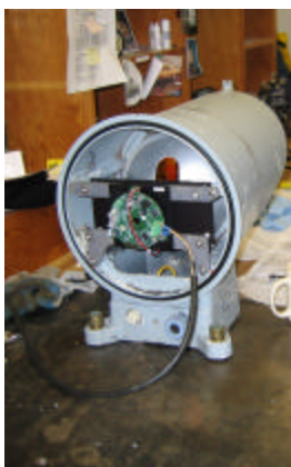
Installed ALS-240/1 in FA-240 Range Light
