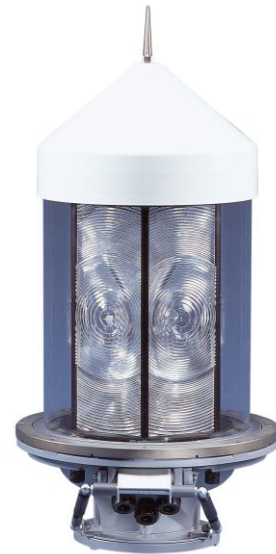
The Tideland TRB-220 rotating beacon for Mombasa is configured with six lenses as required by the flash character and three halogen lamps. ( A high resolution file is available on request)
