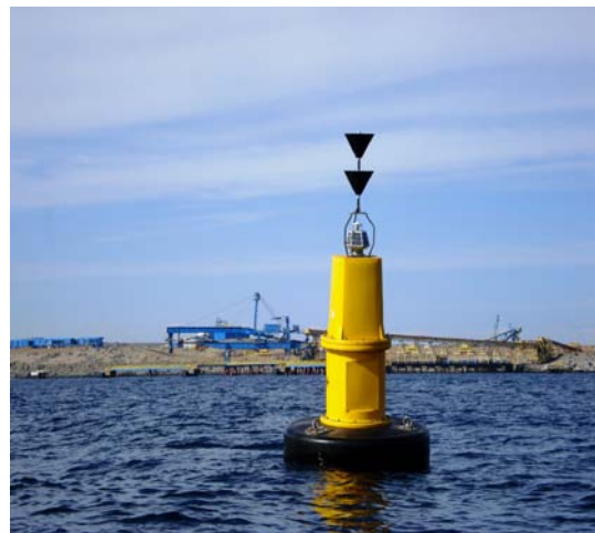
A Tideland SB-2200 buoy equipped with a SolaMAX 140 self-contained LED lantern on station.
