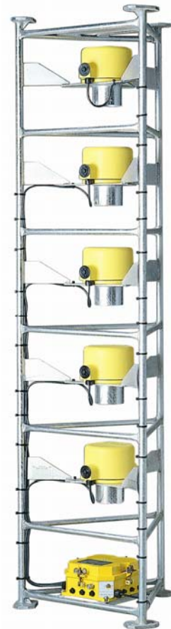
Tideland's AB-560 fog signal incorporates five drivers/emitters producing 133.2 dB at 1 metre equivalent and broadcasting a 360° sound beam in the horizontal plane.
