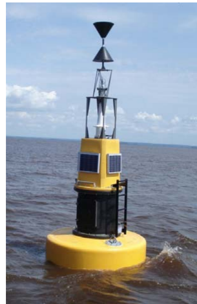
A Tideland SB-2200 buoy configured as a Cardinal Marker and fitted with a SeaBeacon2 System 6 racon and MLED-140 MaxiHALO lantern marks a reef outside the channel into the Port of Soyo.
